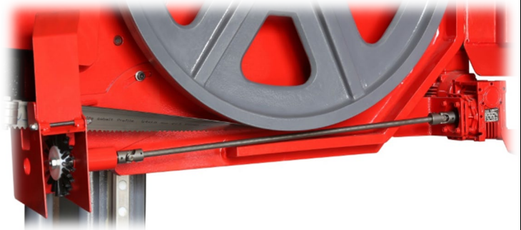
Electrical Motorised Swarf Brush
