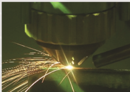
laser cladding process on turbine blades
