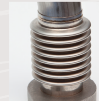
cw laser welding of flexible metal bellows with a connecting part made of high-alloyed CrNi-steel
