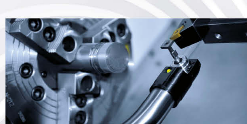
Tool Measuring Device(option): Tool setting device could measure the coordinate of tool profile top automatically so that user can take less time in measuring the tool. Tool abrasion will be compensated automatically.
