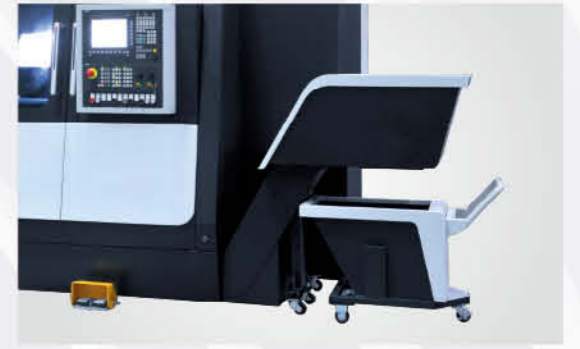
Chip Removal System: There are three types of chip removal modes available for selection: left chip removal, right chip removal and rear chip removal. Cooling pump is a large flow high head. The coolant tank and chip conveyor are separated from the main machine to ensure that the accuracy of the machine shall not be affected by cutting heat.
