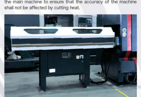
Receiver/Feeder(option): With the rhythm of production, receivers send workpiece to the machining position. Then it picks up a box, spins to the position to get the workpiece and put it into collection box. User can get the workpieces without stopping the machine.
