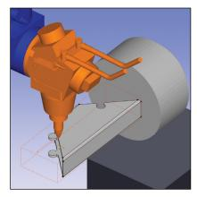
Library of standard shapes In a similar way to tube sections, Radtube supplies a library of parametric hole shapes, again with the option to define 'freeform' shapes; so specialist joint features such as duck tails, clips and key holes are easily added. Holes in the tube are created by generating a solid object to represent the shape, which is then extracted from the tube. The solid can pass through all walls or one wall and can pass through the edge of the section creating a gap.
