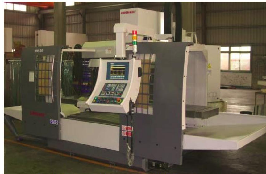
Semi-Enclosed chip guards for VM-28 as standard
