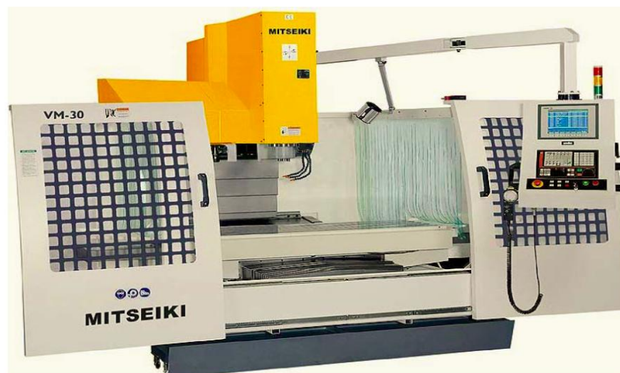
Semi-Enclosed chip guards for VM-30 as standard
