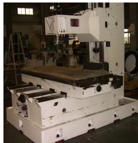
Four-box ways on Y-axis provide exceptional table support
